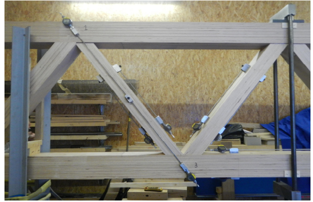
Figure 28: Measuring deformations of diagonals and of the connections.
