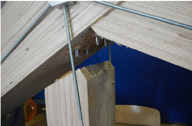
Figure 26: Failure of the steel rods after plastic deformation of more than 5 mm (no pull-out failure = no wood failure)
