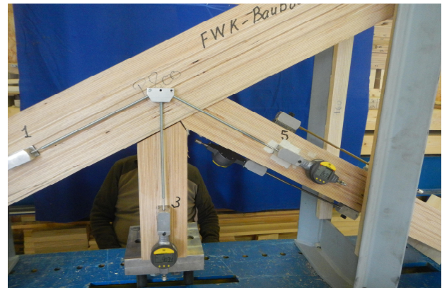
Figure 23: Test specimen of typical connection in a truss with measurement device of tension and compression joint
