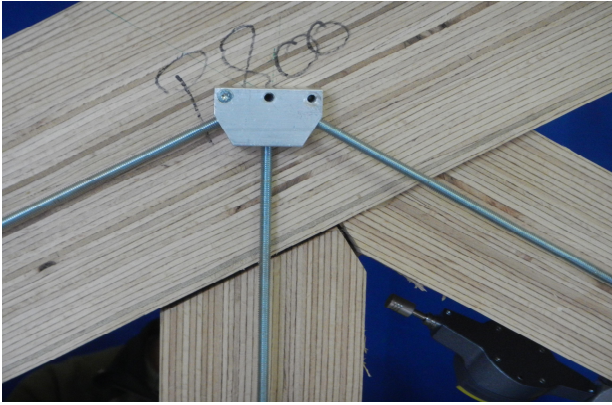
Figure 25: Aspect of connection at the beginning of plastic deformation
