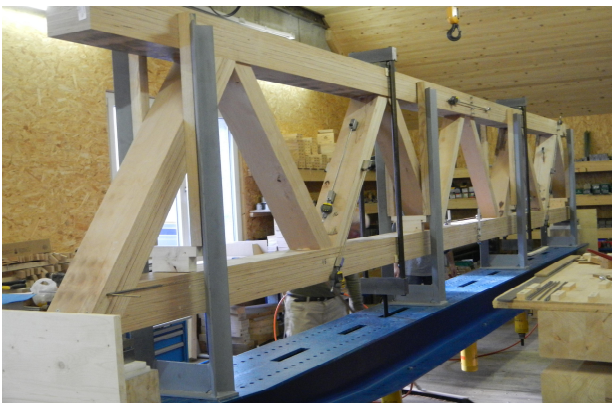
Figure 27: Test of a truss girder with depth of 1 m and span of 7.2 m. Upper and lower cord section 160/180 mm, diagonals with section 100/160 mm. (Built in LVL-beech)
